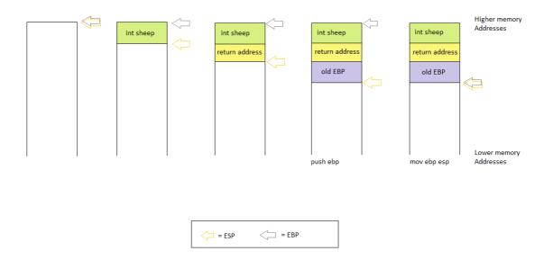
The picture above illustrates what happens when our function main calls the function sheep(1337). First our function arguments are pushed onto the stack in reverse order, which is where we get the green box. It is holding the value 1337. After we finish executing this function we need to know where inside of main we are going to resume execution, this is why we save the return address. This is the yellow box.
