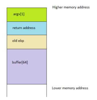
When we call the function strcpy() it will copy the contents pointed to by argv[1] into the contents of buffer. The contents will be copied starting from lower memory addresses and will work their way up toward higher memory addresses.
