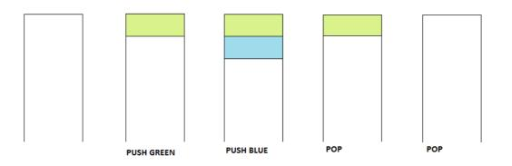
We are storing colored blocks in memory through a series of pushes and *retrieving/removing them* from the stack with a series of POPs. You may not realize it when programming, but you're using the stack all the time!
